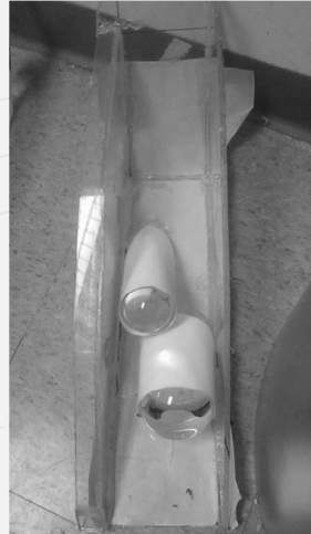
Plastic Framework of Main LED Headlights
